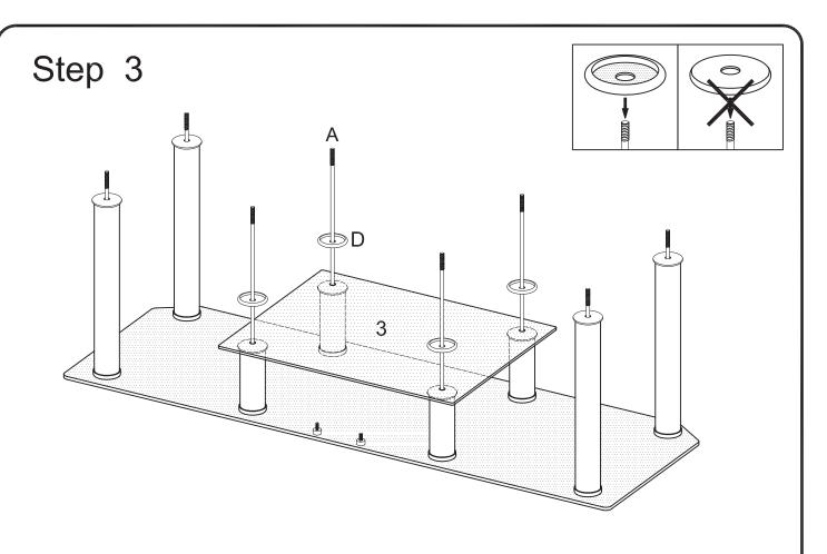
Carefully slide glass (3) into place using middle long rods (A) as guides. Slide decorative rings (D) onto middle long rods (A).
